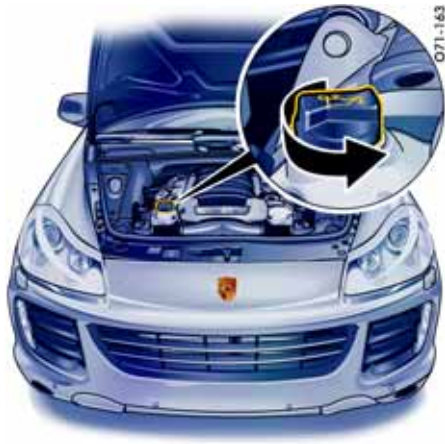
Engine oil filling point on Cayenne S
