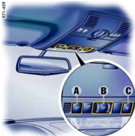
A, C - Switches for reading lights B - Switch for interior light
