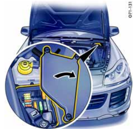
Fuse box in engine compartment
