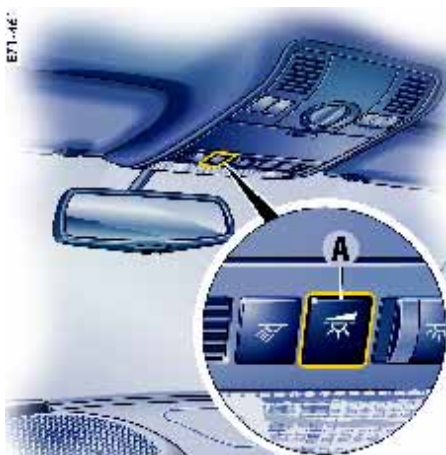
A - Button for dimming the comfort lighting
