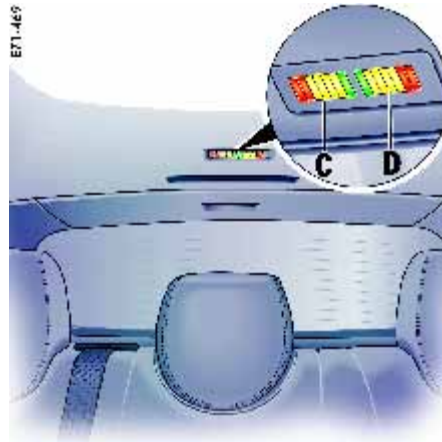
C - Rear display – right monitoring area D - Rear display – left monitoring area
