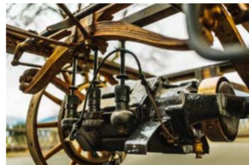
A swinging axle suspension protected the electric motor from impacts
