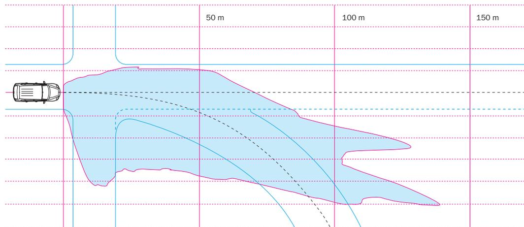
**The stationary cornering light illuminates the turn-off lane; the dynamic cornering light illuminates the bend of the curve**
